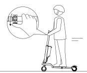
4.Continue to press the thumb shifter to speed up, turn the grip to adjust the direction.
