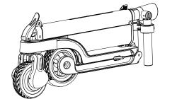
6. Slide fixture outward, Fold the handle.
