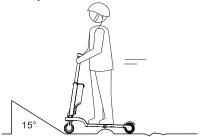
⚠ Be careful of the road with roadblock, sandstone, ponding, mud, wet, ice and snow, slope (angle >15°) stairs, dark area when you are riding.
