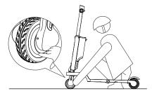
After riding for a long time, the motor hub and disc brake disc would be possible with high temperature. Don't touch them directly to avoid scalding!
