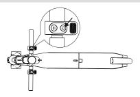
1.Long-press the power button for 2seconds.
