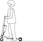
2.Stand on the pedal with single foot, press the acceleration dial, and push the other foot backward.
